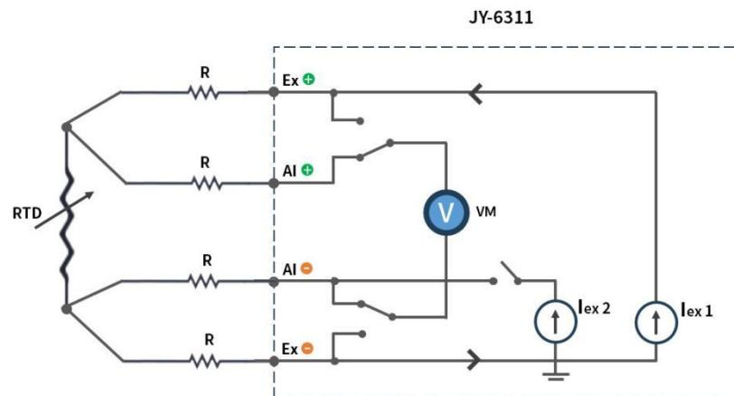
Figure 5 4-wire RTD connection
