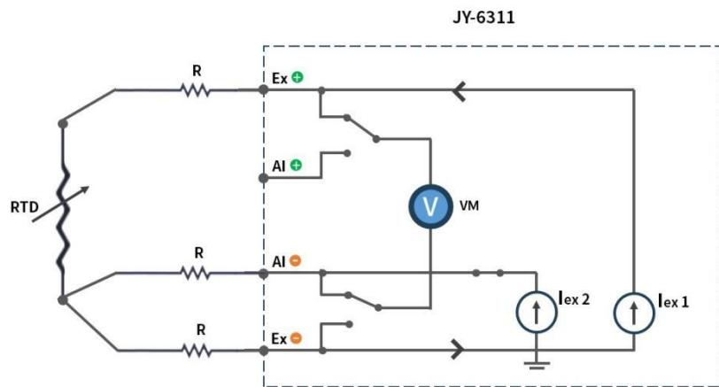
Figure 4 3-wire RTD connection
